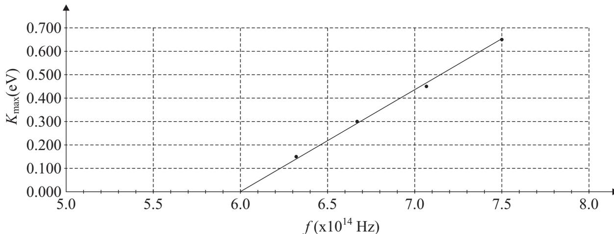
$$(c) \quad m = \frac{\Delta KE_{\max}}{\Delta f} = \frac{(0.65 \text{ eV} - 0.15 \text{ eV})}{(7.50 \times 10^{14} \text{ Hz} - 6.32 \times 10^{14} \text{ Hz})} = \boxed{4.24 \times 10^{-15} \text{ eV} \cdot \text{s} = h}$$
